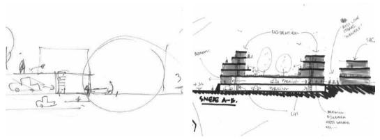
Fig. 2 - Sketch sections made during a design meeting about a mixed programme project to explore the status of 'the alley'. The left sketch highlights this alley as an entry to a lower layer of dwellings. The right sketch elaborates on this. After some scribbling that reflects the discussion, the architect annotated 'low-traffic street - home zone'. © ArchiSpectrum.
